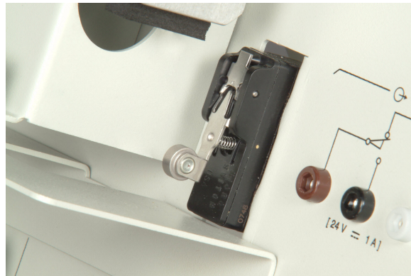
Figure 60. Mechanical limit switch.
